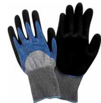
BG191 Cut Resistant Level 5 13 gauge, HPPE shell Black sandy nitrile coating on palm Reinforcement between thumb and index Sewn TPR molds on fingers and back Hook & Loop wrist
