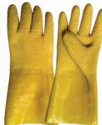
BG407 Latex fully coated Crinkle finish Jersey lining Gauntlet cuff
